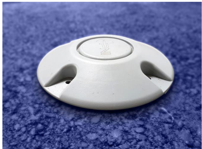
Figure 11: One of the parking sensors placed in the garage facility
