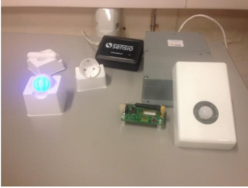
Sensors, gateways from Fibaro/Sensio & Serinus/Tiny Mesh and ATAG appliances located in AAU Lab
